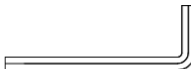
D4. Hexagonal socket wrench 8mm, opposite sides (1PC)
